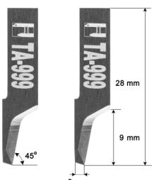
**Materials:** Texon, fiber board with thicknesses up to 3 mm, leather up 6 mm, with the possibility of high cutting speeds. 2.5 mm of radius.
