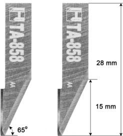
**Materials:** Very rigid materials, thick leather (soles till 6 mm, belts etc), asbestos-free, reinforced graphite, for thicknesses up 10 mm, ideal for small radius.
