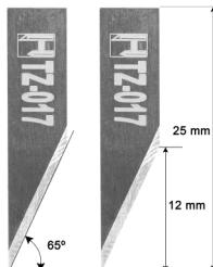
**Description:** Blade for cutting thin materials. The overcut is smaller, but the blade exerts more drag force than the HTZ-16. For best results, use as an oscillating blade.
