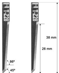
**Description:** Long oscillating blade for soft, thick materials.
